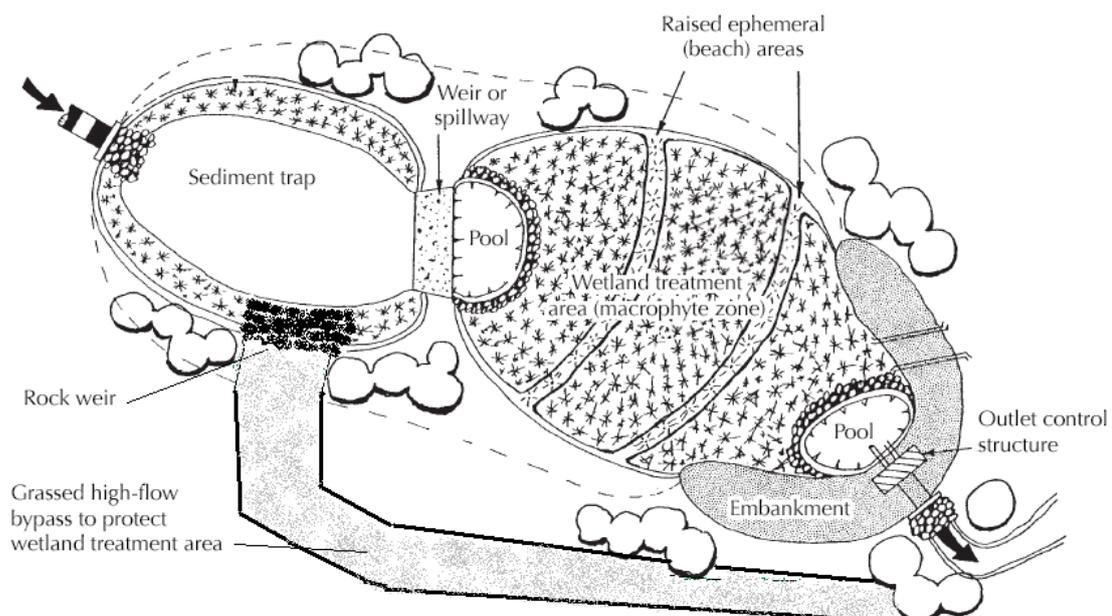
Schematic layout of a sediment trap combined with a wetland system consisting of two separate cells, where a deep trap flows into a shallow wetland. The sediment trap removes coarse sediments, protecting the wetland vegetation from smothering, and the high-flow bypass protects the wetland vegetation by allowing storm flows to pass around the wetland.
