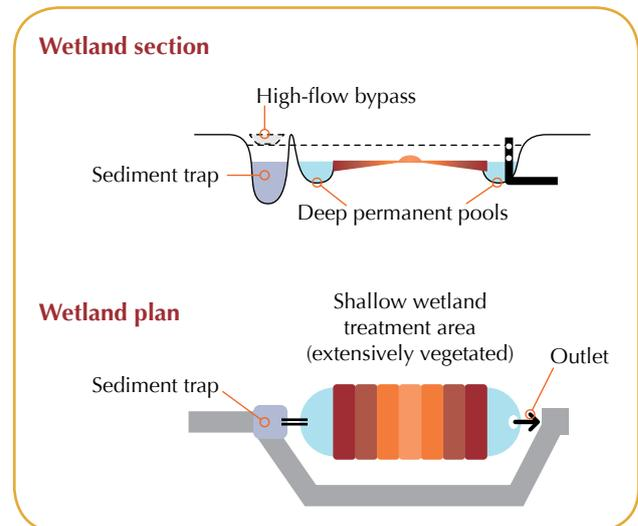
Conceptual layout of a treatment wetland showing sediment trap, high-flow bypass and deeper pools in the main wetland treatment area (Figure based on *Healthy Waterways*, 2006).
