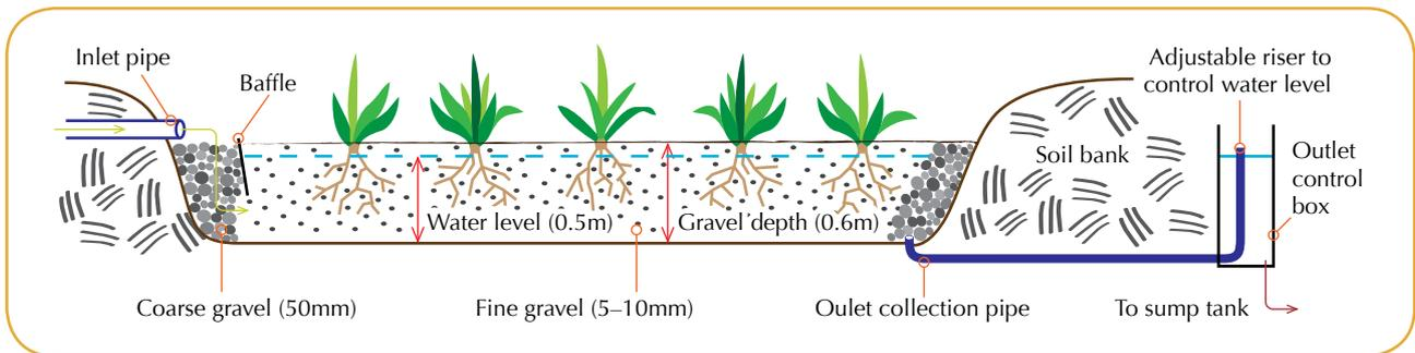
Schematic of a subsurface-flow wetland. (Original diagram courtesy of Dirou et. al, 2003).
