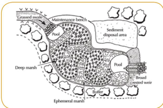
Schematic layout of a surface-flow wetland
