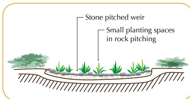
Schematic of a stone-pitched weir outlet that enables vegetation to be incorporated in the design. (Figure courtesy Melbourne Water).
