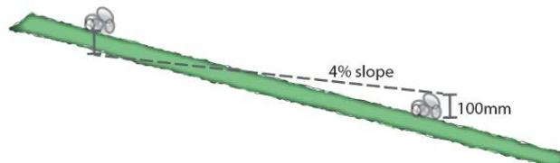
Figure 3 - Rock check dams on base of steep swales/drains
