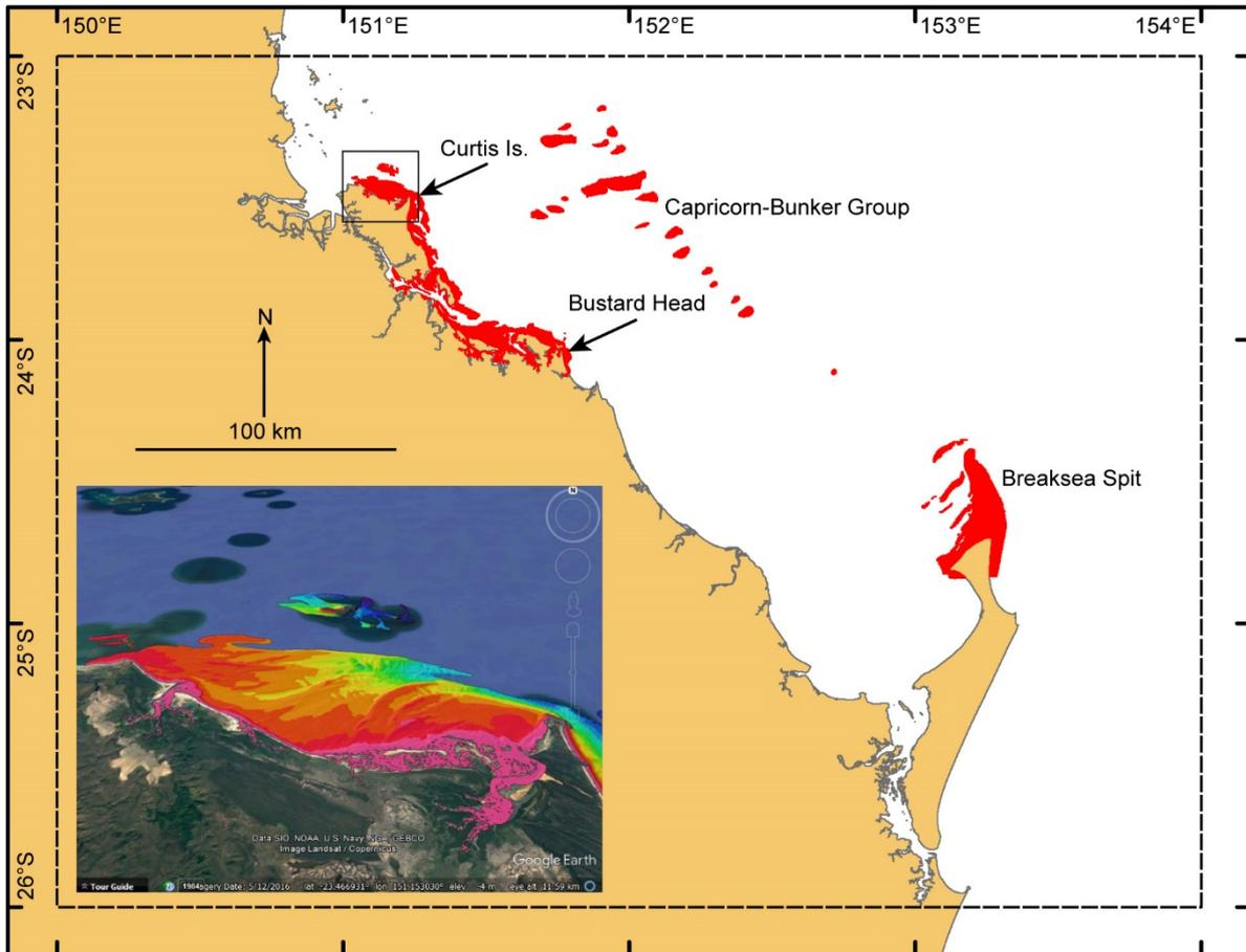
Figure 8 Satellite derived bathymetry (SDB) source data coverage. Inset shows typical EOMAP-supplied SDB data for Curtis Island area as oblique view in Google Earth.
