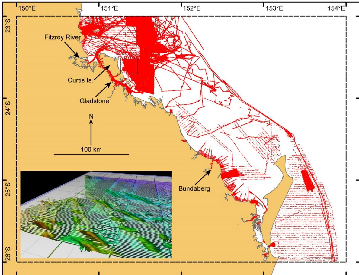
Figure 4 Singlebeam echosounder source data coverage. Inset shows typical AHS-supplied HI282\_Gladstone survey as oblique view in Fledermaus software.
