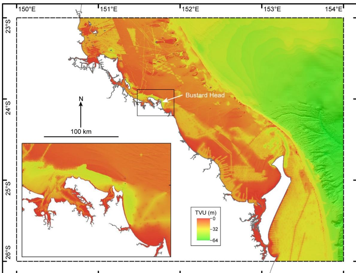
Figure 188 Histogram-stretched view of the Total Vertical Uncertainty grid. The inset shows the Bustard Head area and the relatively larger TVU values for the EOMAP SDB source data.
