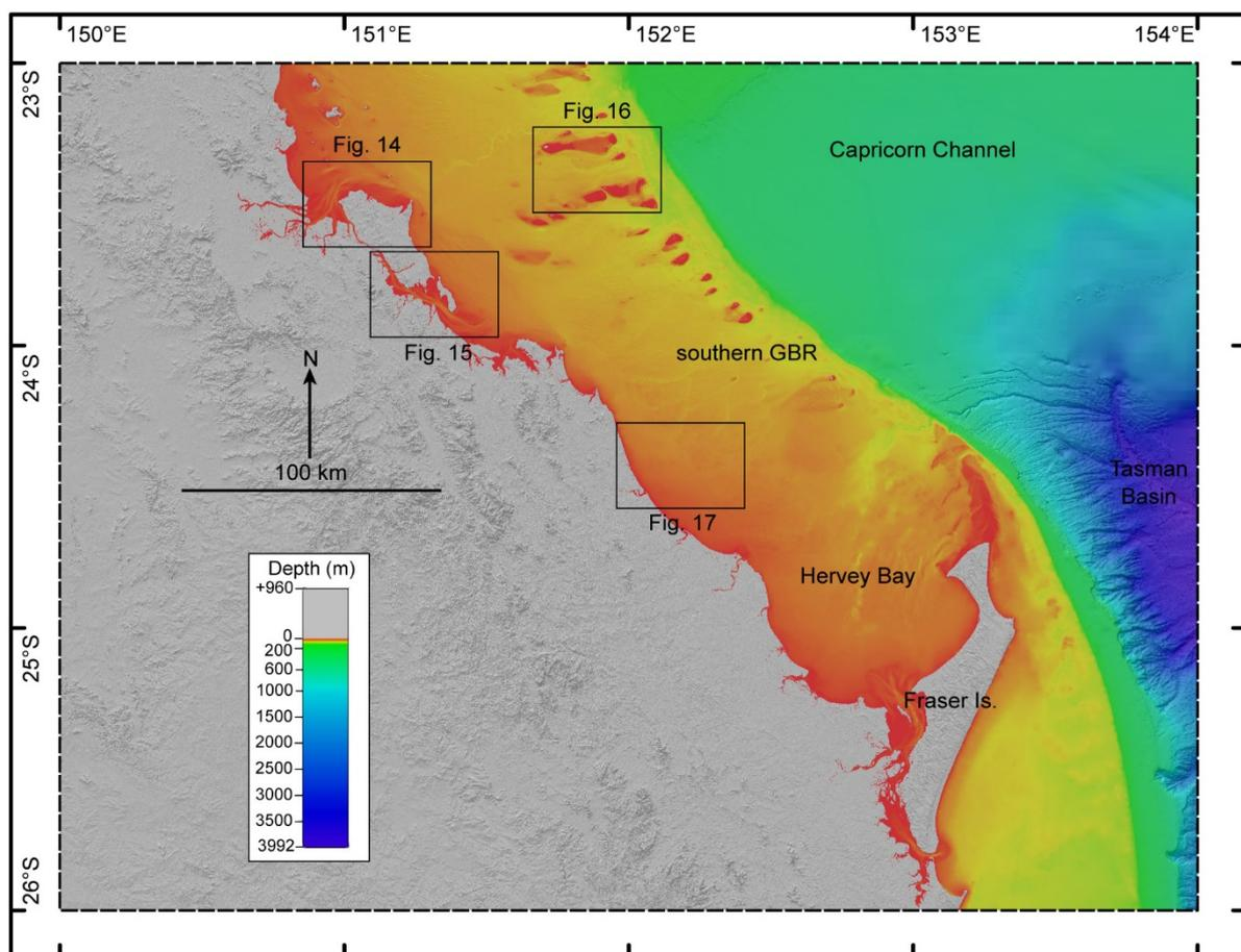
Figure 13 Coloured hillshade view of the ceq30 bathymetry grid, shown with vertical exaggeration x6, sun azimuth 315°, and sun angle 51°. Boxes show locations of Figs. 14-17.
