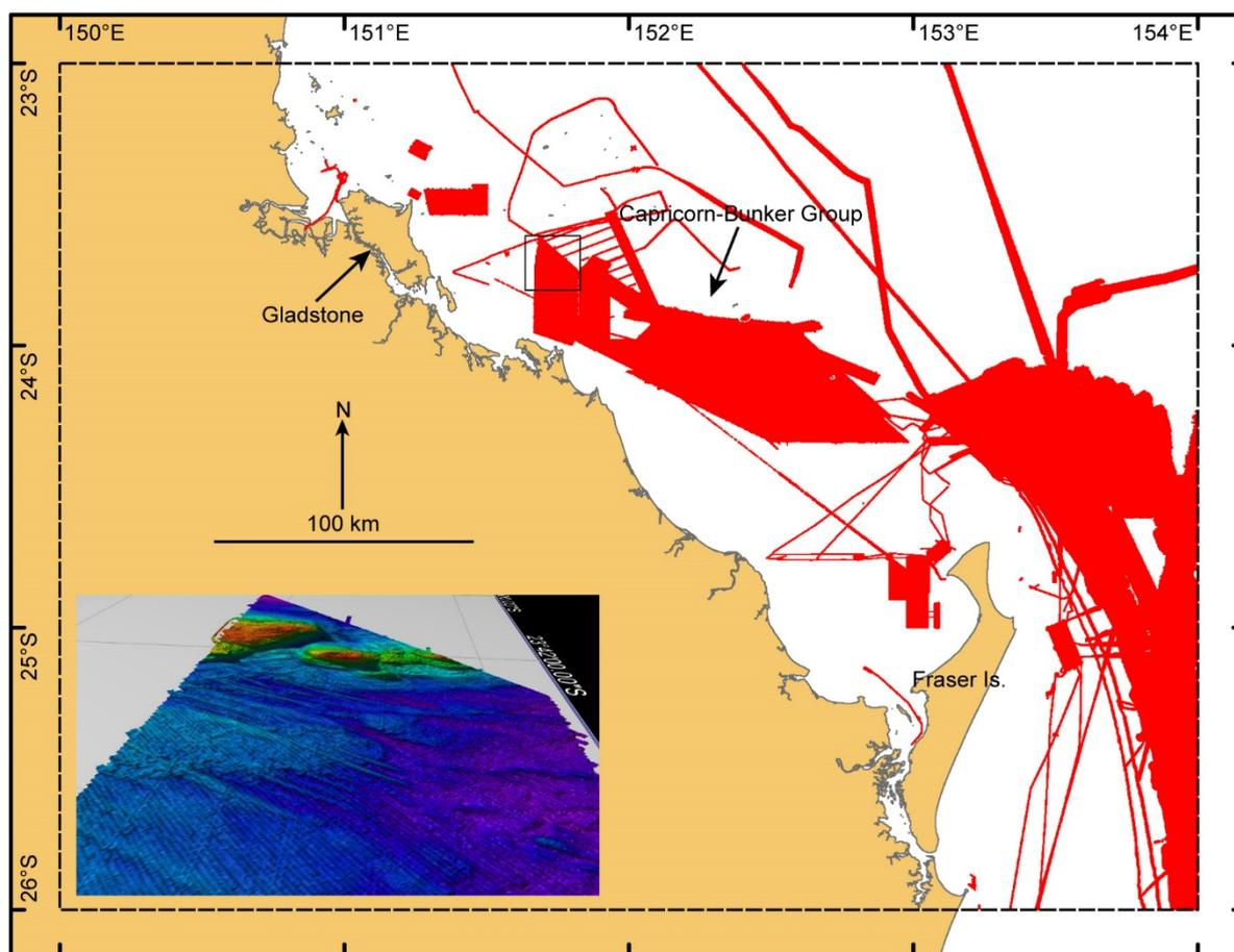
Figure 3 Multibeam echosounder source data coverage. Inset shows typical AHS-supplied HI442\_ApproachesToGladstone survey as oblique view in Fledermaus software.
