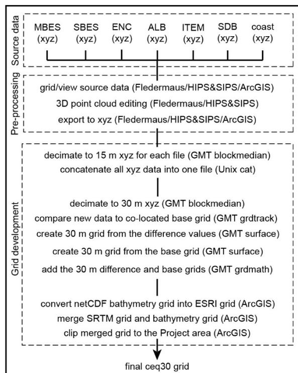
Figure 11 Processing scheme used to develop the ceq30 bathymetry grid.
