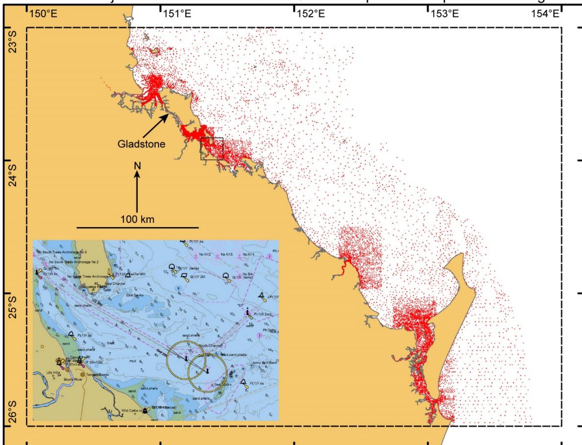
Figure 5 ENC spot depth source data coverage. Inset shows typical ENC S-57 tile AU424151\_Keppellsles near Gladstone Harbour using the ESRI S-57 viewer in ArcMap.
