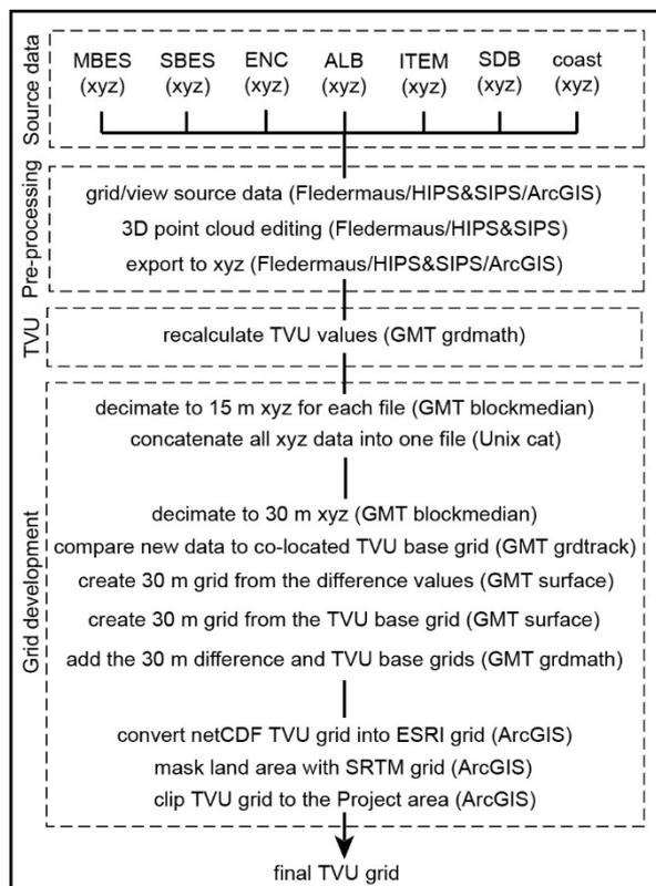
Figure 12 Processing scheme used to develop the TVU grid.
