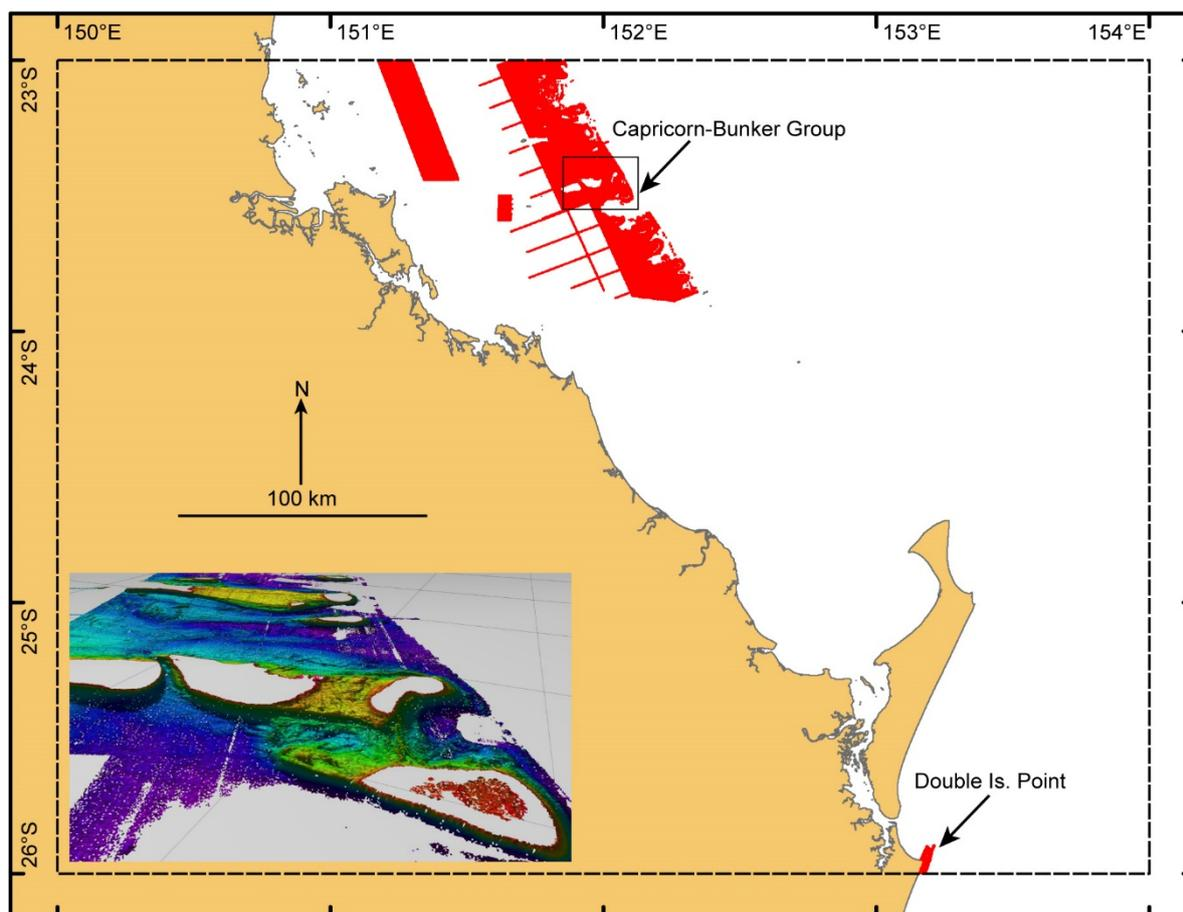
Figure 6 Airborne lidar bathymetry source data coverage. Inset shows typical AHS-supplied H1199\_CapricornGroup LADS survey as oblique view in Fledermaus software.
