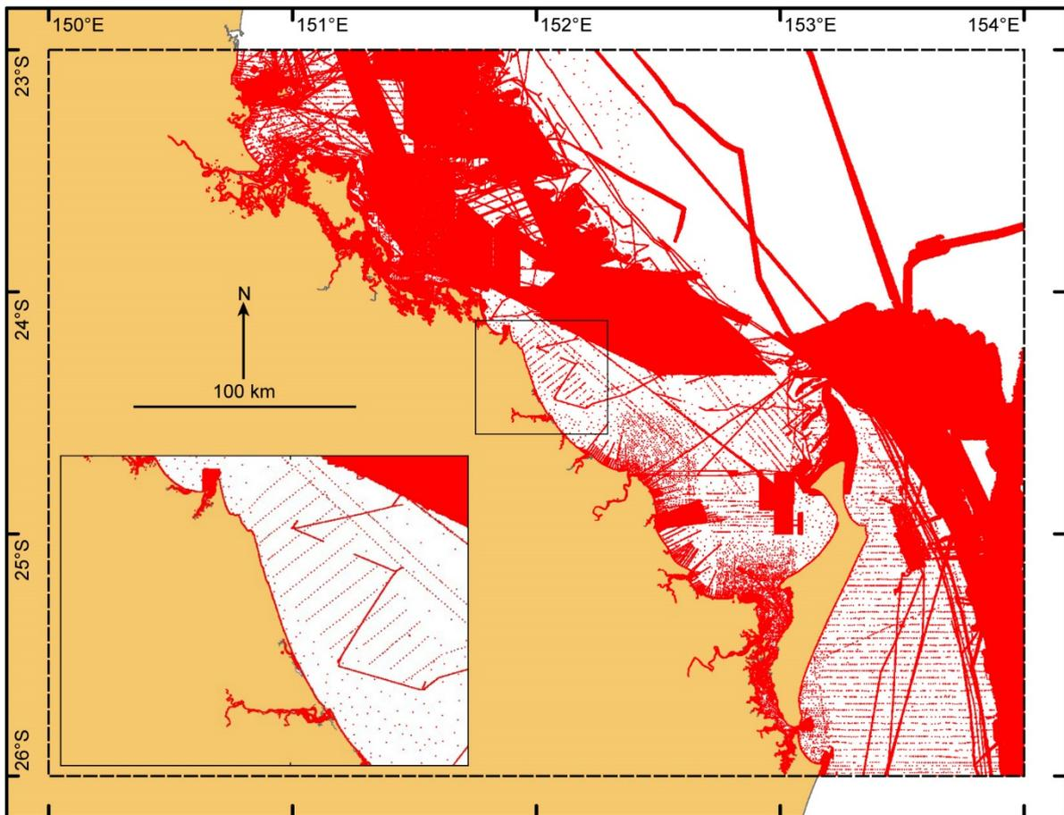
Figure 199 All source data coverage. The white areas indicate the lack of source digital data. Inset shows close-up of source data coverage near Baffle Creek. Also see Fig. 17.
