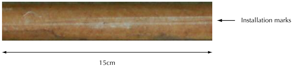
Figure 6. Narrow strips of ferrihydrite paint removed on installation
