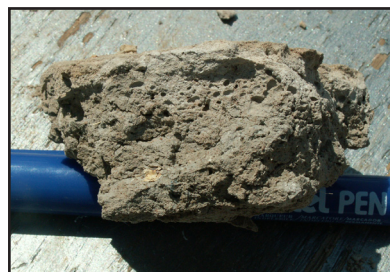
Figure 1. Vesicular structure Very high surface temperatures boil the water inside the soil pores, which evaporate quickly leaving small voids
