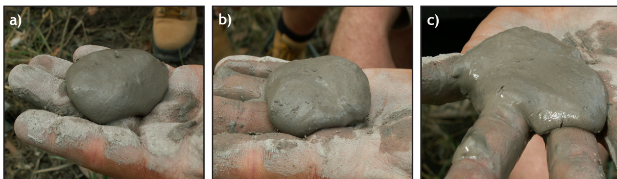
Figure 1. Dilatant soil a) When squeezed into a ball water is held in the soil particles and does not flow out of the soil b) Upon releasing the ball, water quickly appears on the soil surface c) a few seconds later soil particles lose cohesion and water flows out of the ball
