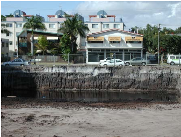
Plate 3 Unconsolidated Pleistocene marine quartz sand deposits with organic staining, Maroochydore (Land Zone 2)
