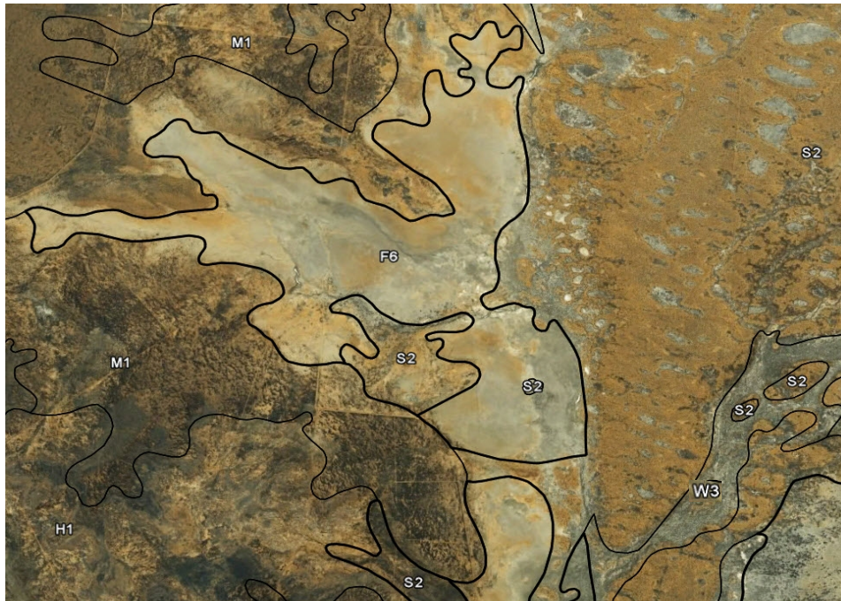
Plate 25 Wind-blown sand plains (S2) of Land Zone 5 overlie paleo-alluvial clay plains (F6) of Land Zone 4 south of Winton.
