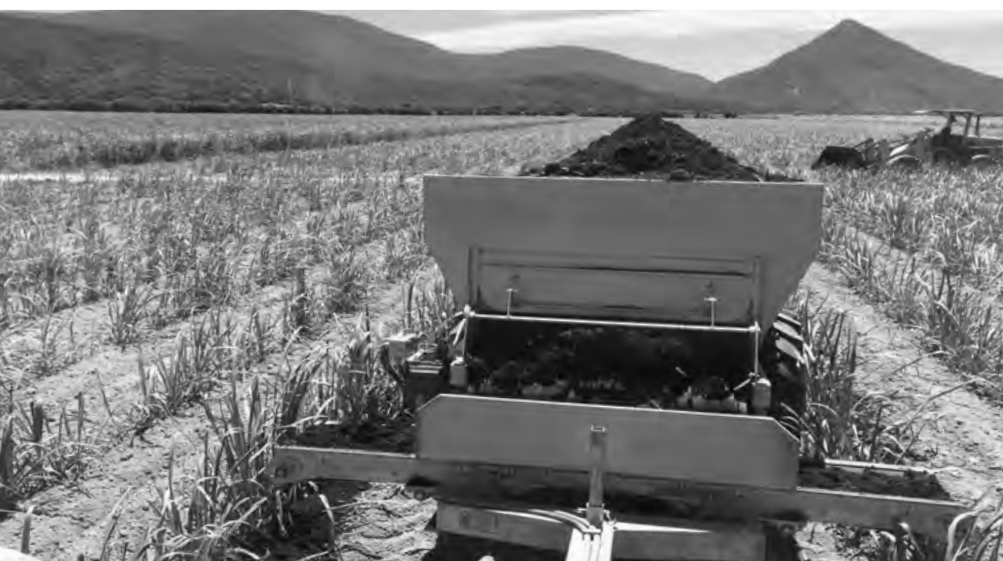
CANEGROWERS Cairns Region purchased a three-row variable rate applicator which is available to members who wish to achieve sustainable practice change around mud, ash and/or compost application.
