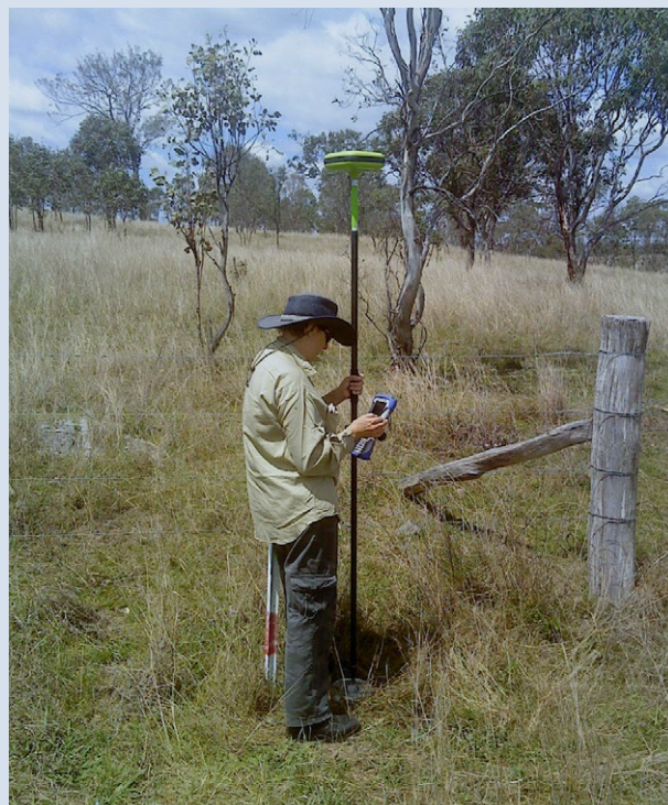
Figure 10 Using Real Time Kinematic (RTK) technology to collect cross-sectional information to assist in determining down-out values.
