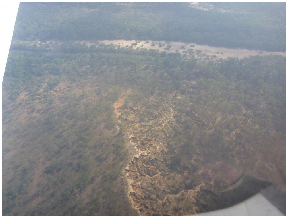
Plate 9. Aerial view of severe gully erosion adjacent to the Palmer River (ml_r00078).
